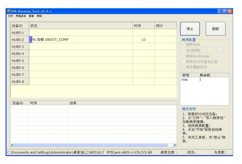
8. After about 5-6mins the process will finish and hit 100%. Then you press stop and plug the box out, and connect box with power to turn it on see if the box working normal. The first boot will take about 5mins.
