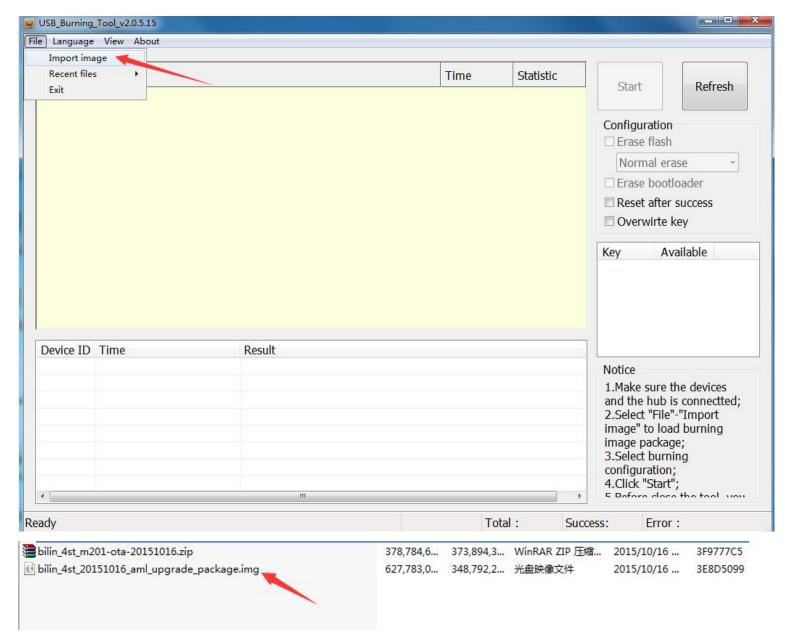
4.After loading file finished you need to connect USB cable to the computer USB port (if you are using desktop computer to do this you must connect the cable from the computer backside USB port as it can providing you full 5V voltage to avoiding failure)
